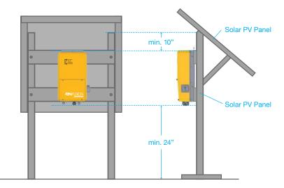
Figure 1: Blender 2500 Mounting Clearances
