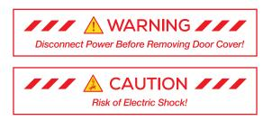
Before performing any service or maintenance inside the controller or when connecting or disconnecting any wires, **DISCONNECT the power** and **WAIT 90 seconds** to allow the capacitor bank inside the controller to discharge to a level below 50V.
