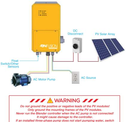
the positions of any two of the three motor wires. It will change the of rotation and it should start pumping water!
